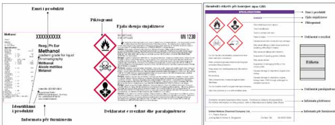
Fig. 10: Labelling of hazardous substances
