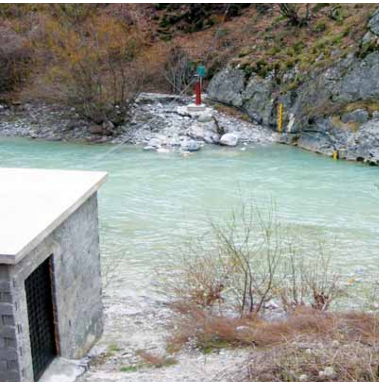
Photo: Hydrometric station in the Bistrica e Pejës river – Gryka e Rugovës and the elevator system for water flow measurement
